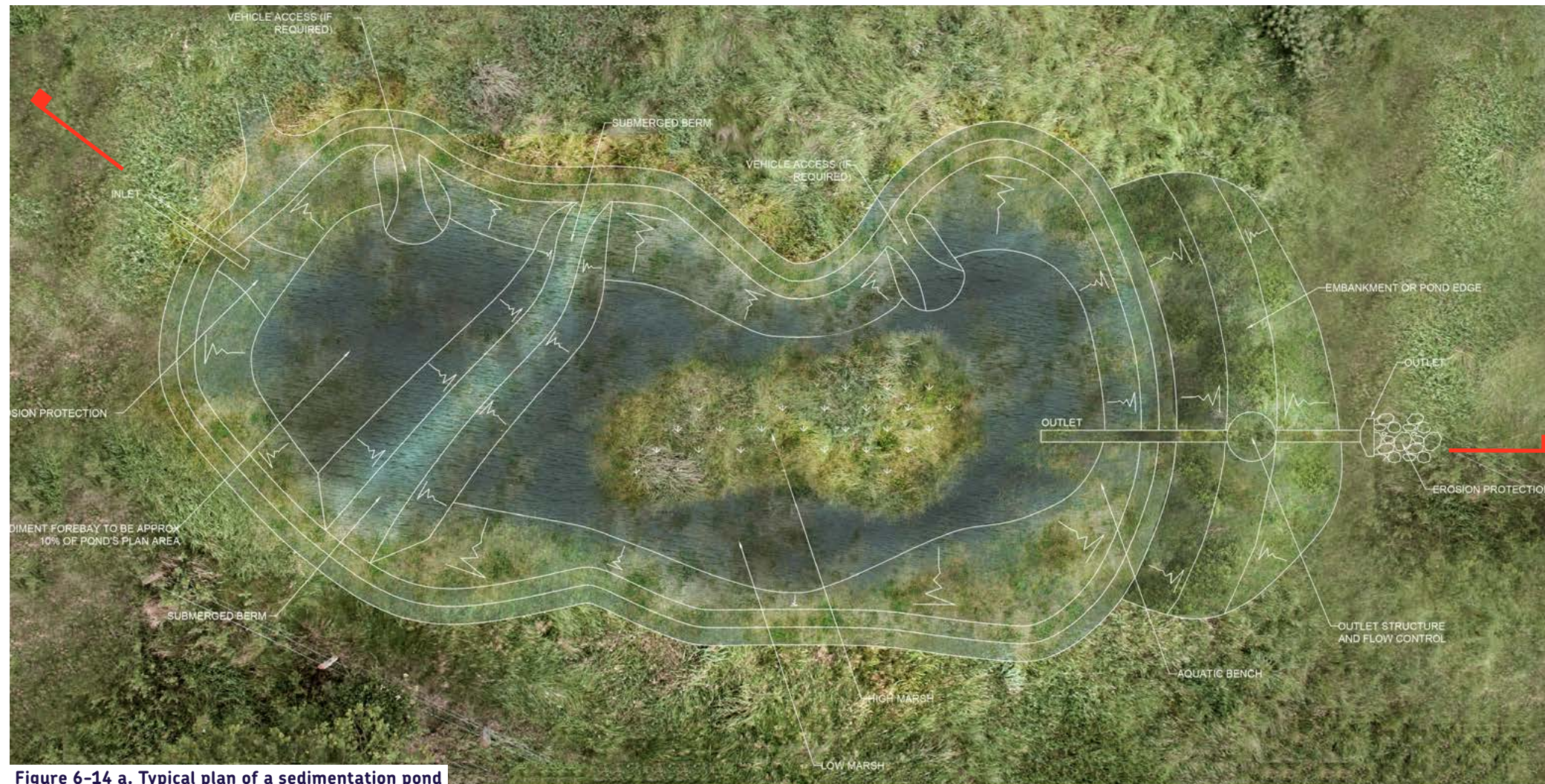
Figure 6-14 a. Typical plan of a sedimentation pond
